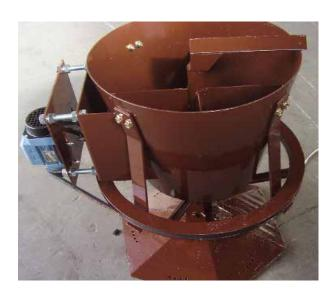
The Silos Córdoba's grain spreader is an optional accessory that gently distributes the grain throughout the silo using gravity. The force of falling grain against the spreader avoids the accumulation of grain at the center of the silo, thus ensuring full storage capacity.
