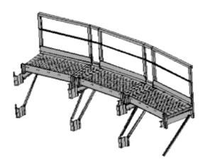
A perimeter catwalk for access and maintenance is placed at the top of the silo cylinder. It includes transit floor.
