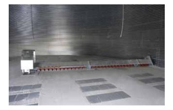
Silos Córdoba **sweep augers** adapt to our silo diameters and can be complemented with accessories that enhance emptying by eliminating all existing residue between the sweeping machine and the ground. Complies with the ATEX standard for work inside a silo.
