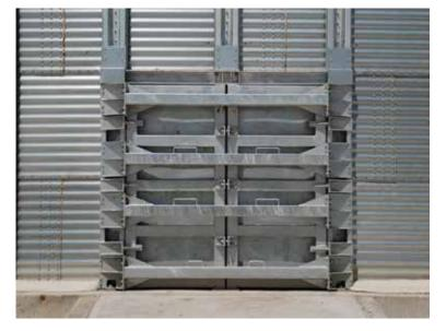
**Bobcat door** opening is ideal for high-capacity silos which are unloaded using light Bobcat machinery so the product residual slope is emptied. It is made with a rigid frame featuring pillars that transmit the loads to the ground and horizontal reinforcements.
