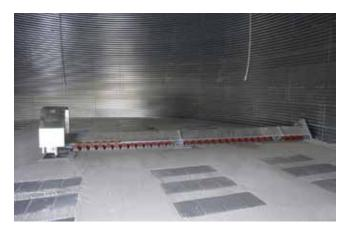
Silos Córdoba sweep augers adapt to our silo diameters and can be complemented with accessories that enhance emptying by eliminating all existing residue between the sweeping machine and the ground. Complies with the ATEX standard for work inside a silo.
