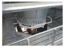
The **vibrating bottom** helps to unload the products stored in hopper silos with poor flow characteristic like flour, granulated poppy, small shells, carbonate, soya beam meal, etc. Recommended for silos with a 60° cone that is reinforced to support the vibration. System is available in different diameters and we adapt it to different silo outlet dimensions.
