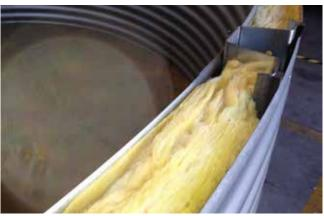
Double sheet plus insulation material: Insulation material is added between sheets. The most common materials are polyurethane foam and fibreglass wool.
